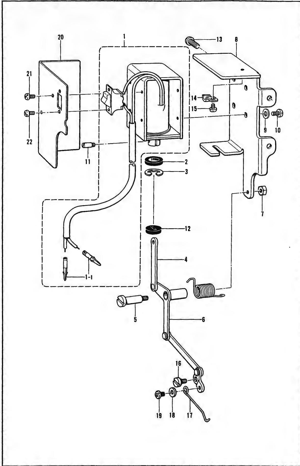
N. 糸扱い関係 / Thread wiper mechanism / Fadenspannvorrichtung /
