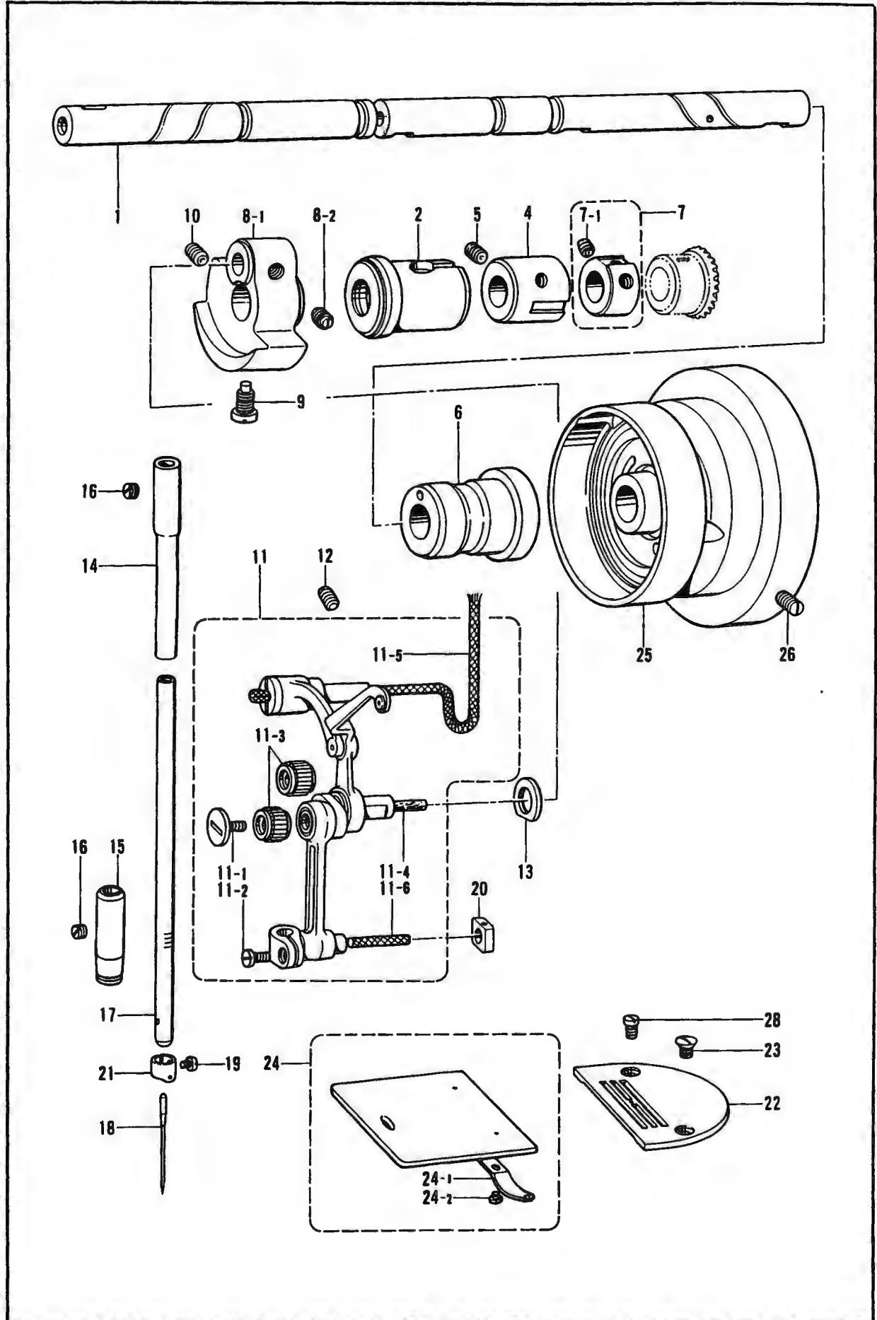
C. 針棒天ビン関係 /Needle bar and thread take-up mechanism /Nadelstangen-und
