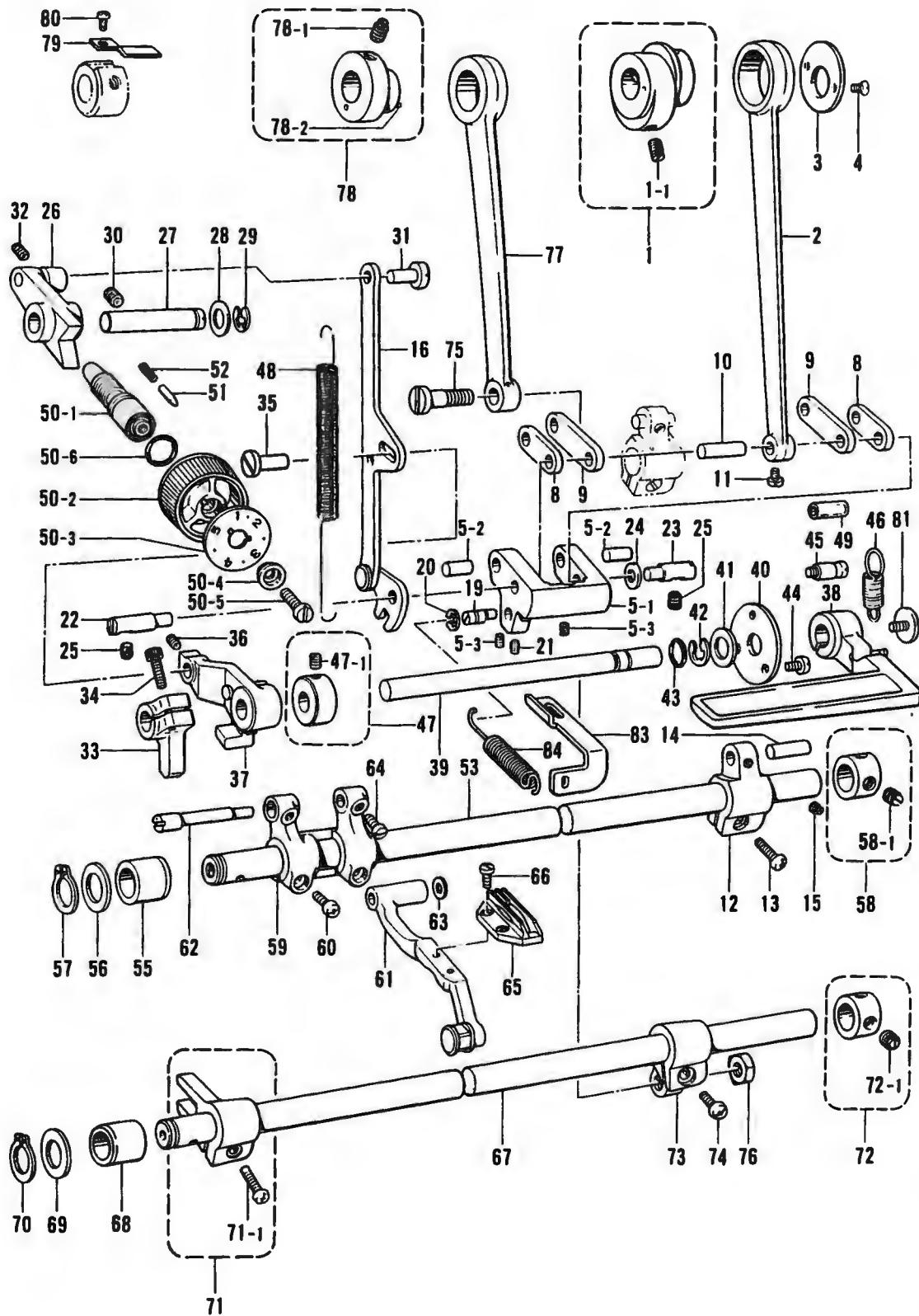
E. 送り関係/Feed mechanism/Transportvorrichtung/
